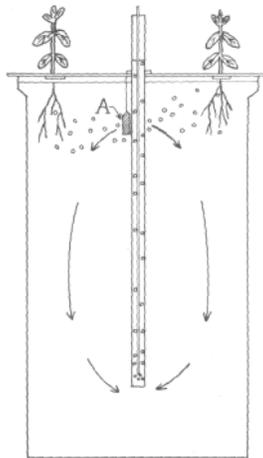
*Fig. 1. Sketch of solution culture apparatus showing position of plant, aerator, and inoculum bag (A).*
