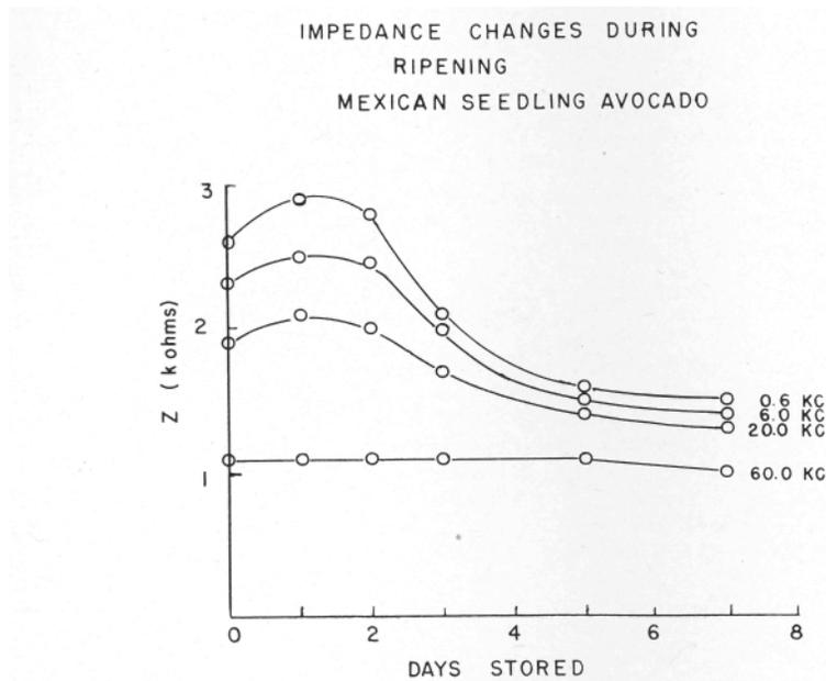
Figure 1. Change in impedance of the avocado fruit during ripening.
