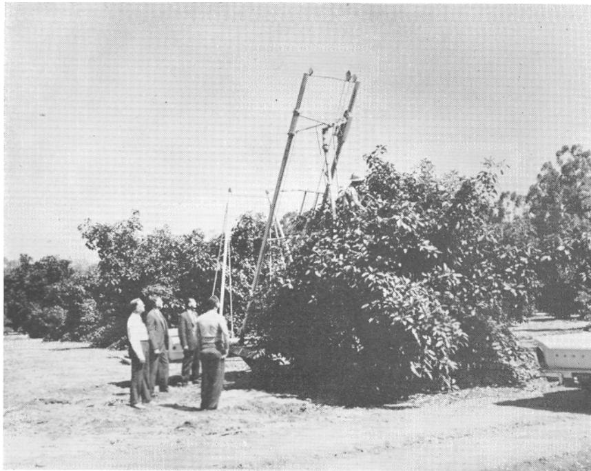
FIGURE 1. Demonstration of fruit picking machine by Dan Seamount, Assistant Specialist, Agricultural Experiment Station, Riverside. Mr. William Cowan and Mr. Phil Newman of Calavo, Gene Dagerman of Space Equipment Corporation, and Mr. Wally Wright of The Irvine Company are observing the test. The operator is shown with his swing seat swung to the left so that he may work directly up against fruit bearing branches.
