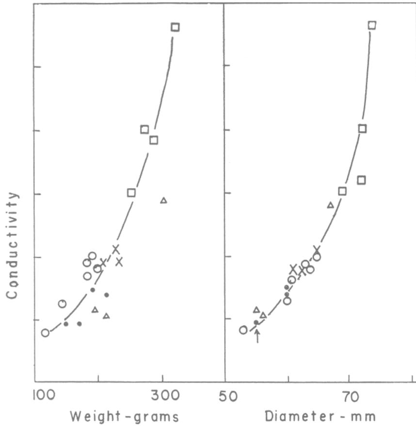
FIGURE 3. High frequency impedance measurements in avocados with fruit in contact with insulated ground electrode. o-Hass; x-Ryan; z-Iwo; y-Dickenson; k-Unidentified. Conductivity is in arbitrary units.
