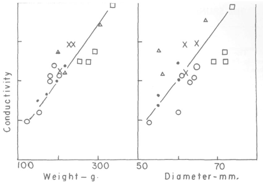
FIGURE 4. High frequency impedance measurements in avocados with fruit contacting insulated live electrode. See Figure 3 for identifications.
