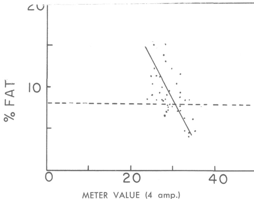
FIGURE 1. Correlation of impedance meter readings and oil content of avocados in field tests. Impedance is given in arbitrary units.
