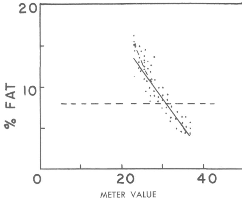
FIGURE 2. Correlation of impedance meter readings and oil content of avocados under laboratory conditions. Impedance is in arbitrary units.
