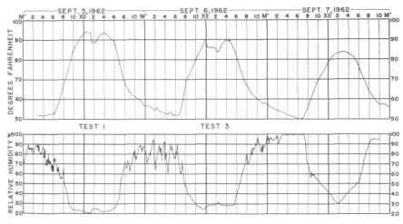
Figure 2. Hygrothermograph record showing air temperature (upper curve) and relative humidity (lower curve) changes in degrees Fahrenheit and per cent respectively for tests 1 and 3.
