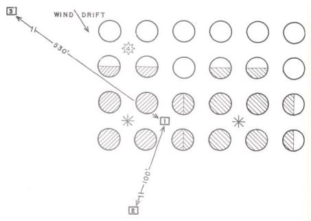
Figure 1. Location of sprinklers (\*), microclimate stations (1, 2, 3), anemometer (4) and portions of trees wet during sprinkler tests (shaded).
