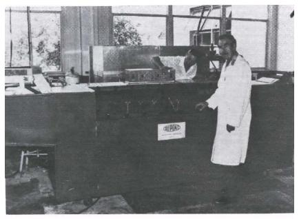
Figure 1. Equipment used in freon freezing of fresh peeled and halved avocados.
