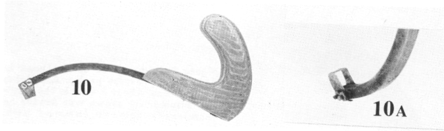
Figures 10 to 13, necked peelers. Fig. 10 (close-up in 10A), curved neck and hook handle. About 3/8 inch. Consensus: Two men said this was the best tool used, while the other man rated it with #9 as tops. The only possible improvement suggested was a "V" attachment on the cutting head to ream out remaining bark from limb depressions.
