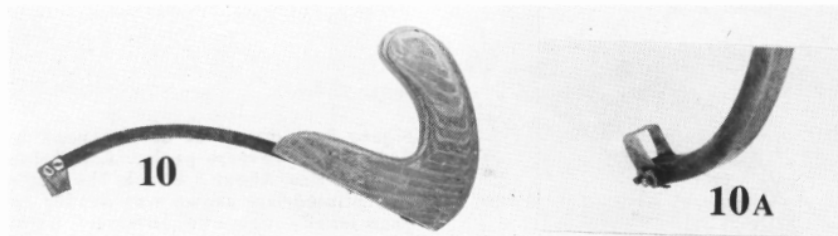
Figures 10 to 13, necked peelers. Fig. 10 (close-up in 10A), curved neck and hook handle. About 3/8 inch. Consensus: Two men said this was the best tool used, while the other man rated it with #9 as tops. The only possible improvement suggested was a "V" attachment on the cutting head to ream out remaining bark from limb depressions.
