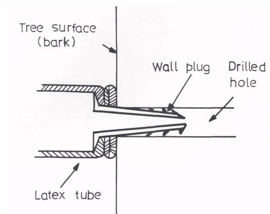
Figure 1. Schematic presentation of the method by which the latex tube is connected to the tree.
