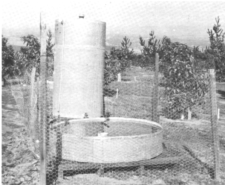
U.S. Class Pan A Evaporative Pan — instrument measures water evaporation; measurements taken regularly for purpose of calculating water consumption by avocado trees.
