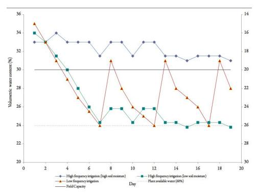
Figure 18. The influence of high and low irrigation frequencies on soil aeration. Total porosity = 50%; FC = Field capacity; AWD = Available water depletion.
