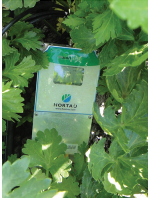
Figure 6. Realtime tensiometric moisture measuring. By monitoring soil moisture in the root zone, irrigation can be applied when water is needed and stopped when moisture reaches the rootzone.
