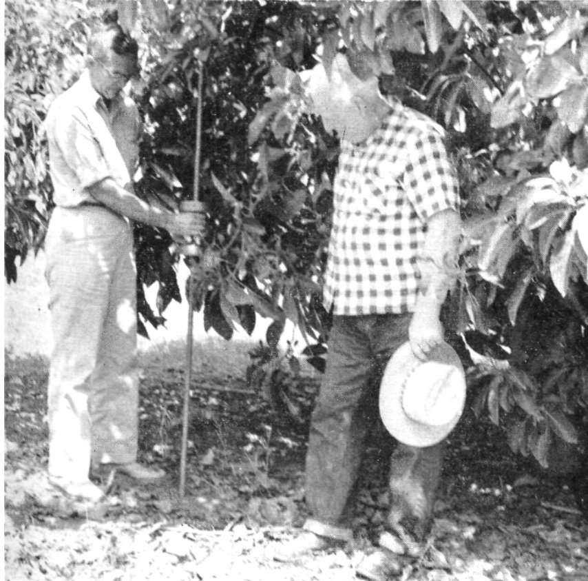
Figure 1. Tensiometers were installed just inside but fairly near the tree dripline.
