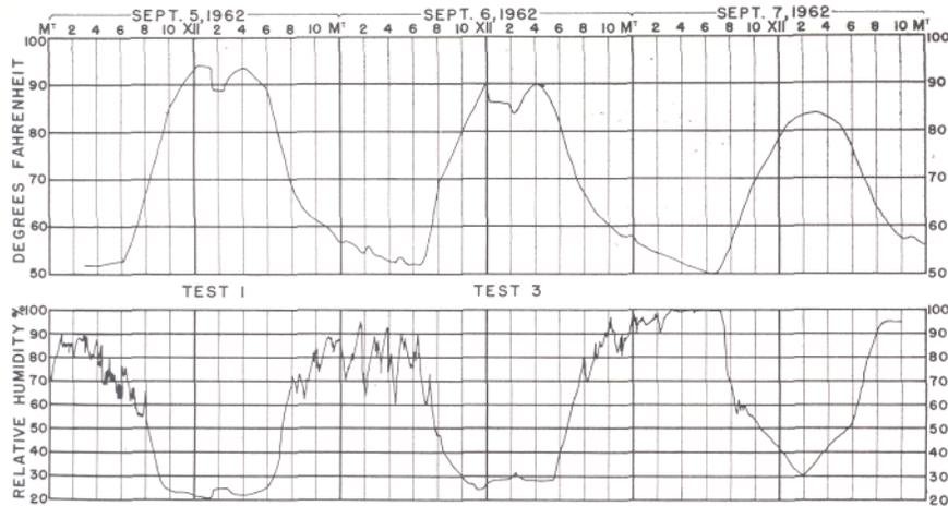
Figure 2. Hygrothermograph record showing air temperature (upper curve) and relative humidity (lower curve) changes in degrees Fahrenheit and per cent respectively for tests 1 and 3.
