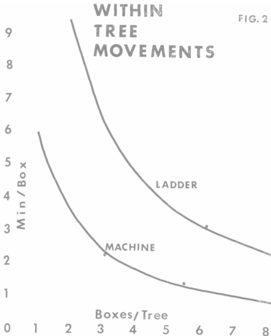
For example, at 7 boxes per tree the distance between curves is 1.7 minutes while at 3 boxes it is about 4.0 minutes. If this is the case for movements within the tree, the machine advantage increases as the yields per tree become smaller.
