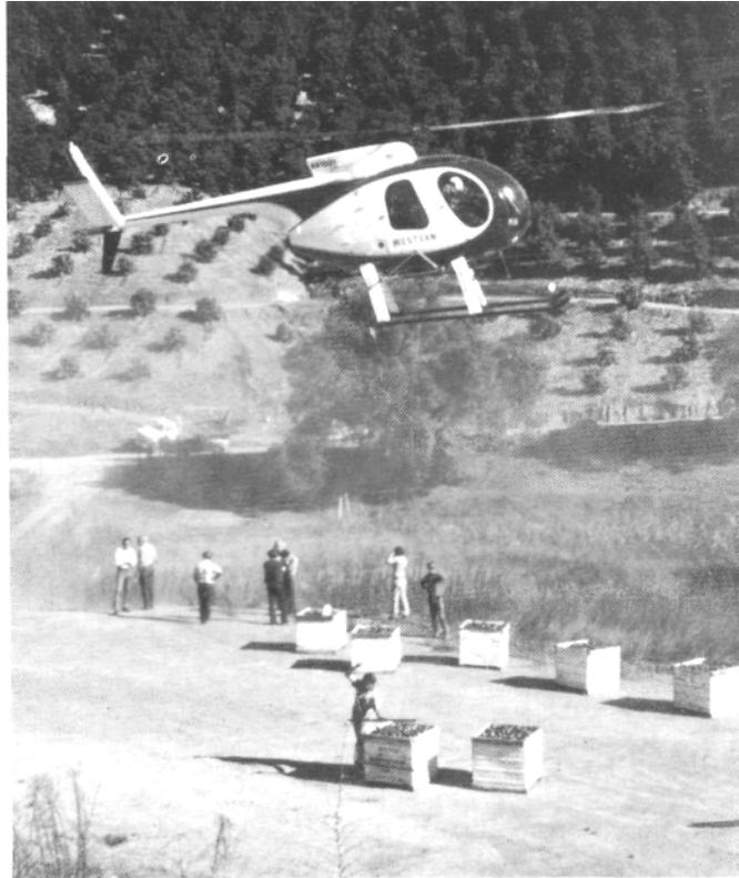
FIGURE 7—Helicopter used to remove full picking bins from steep hillside orchard to a truck loading area within the orchard.
