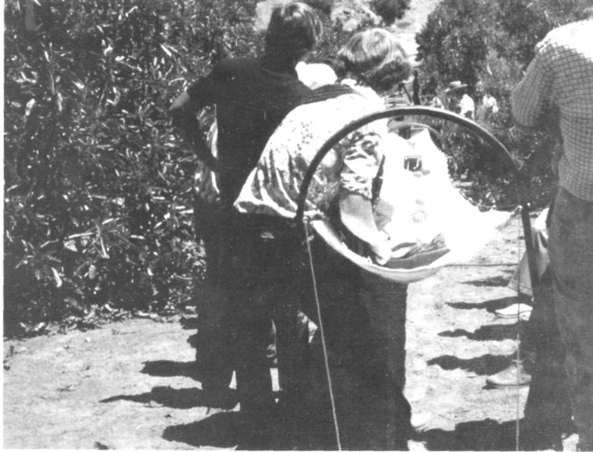
FIGURE 5—"Fruit Chute" set up on a steep hillside avocado orchard. Pickers dump fruit from their picking bags onto the canvas chute, and fruit then rolls down into a large picking bin.
