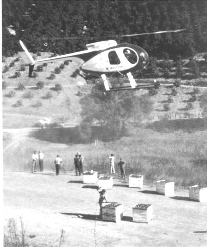
FIGURE 7—Helicopter used to remove full picking bins from steep hillside orchard to a truck loading area within the orchard.
