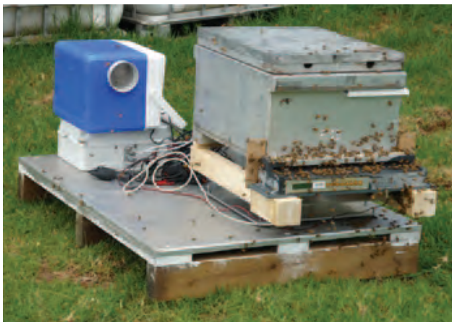
Monitoring the arrival of a swarm of bees to a bait box instrumented with cameras and weight, temperature and relative humidity sensors in controlled trials
