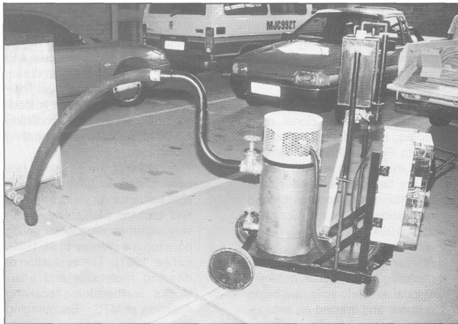
FIG 5. A mobile electrode boiler.
