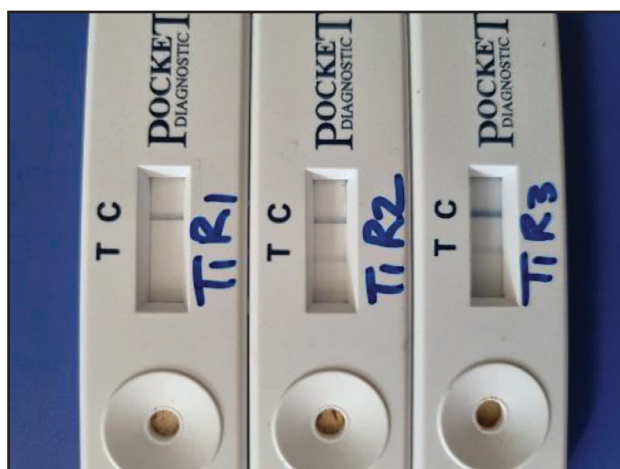
Figure 9: Positive (two vertical stripes) and negative (one vertical stripe at C) reactions observed with the pocket diagnostic lateral flow device for the presence of Phytophthora in roots displaying symptoms of Phytophthora root rot.
