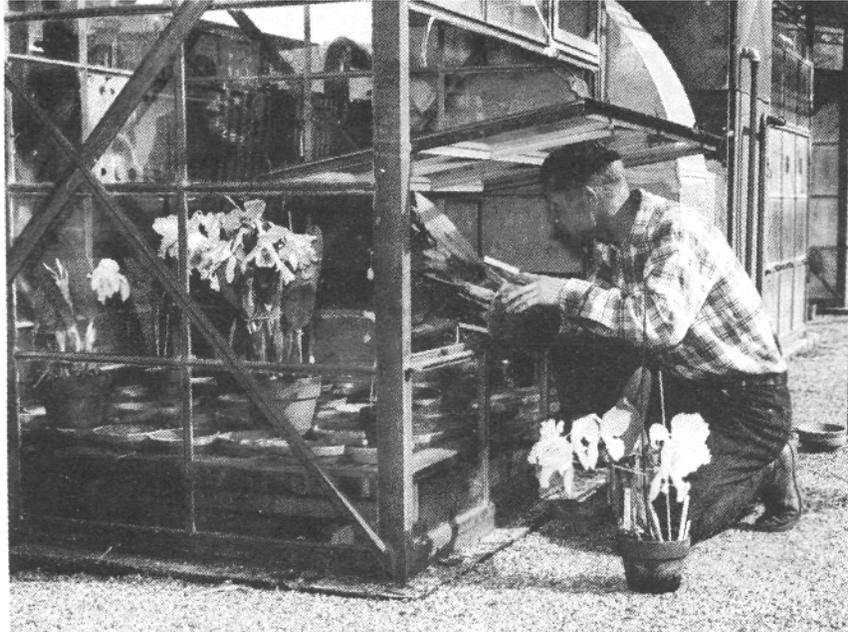
*Close-up of glass chamber used in study of smog effects on plant life, at Citrus Experiment Station, Riverside, Calif.*
