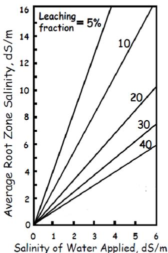
Figure 2. Estimation of percent leaching fraction required to maintain specific root zone salinity. For avocado, the  $EC_{sw}$  should be maintained as low as possible as avocado roots cannot extract water above a value of 4 dS/m. If the irrigation water has an  $EC_{iw}$  of 1, then a minimum leaching fraction of 10% is needed to maintain the average root zone salinity at a value of 2.5. Increasing the leaching fraction to 20% reduces the average root zone salinity to 1.8 dS/m.
