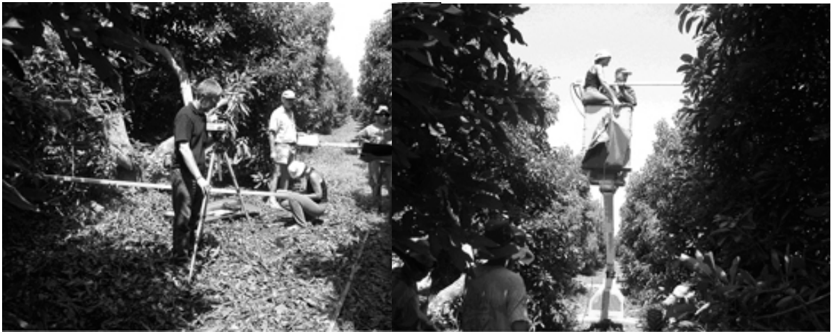
Figure 2 – The BFS held by Dr. Broday coupled with the SunScan probe (left) during measurements of light intensity in different heights, using a 'cherry picker'.
