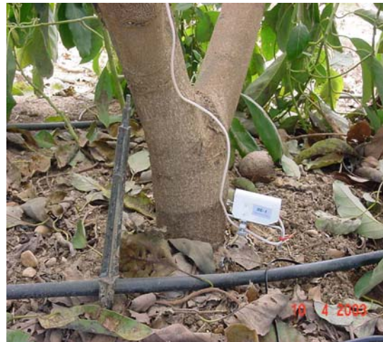
Fig. 1. Electronic trunk dendrometer device on an avocado tree.
