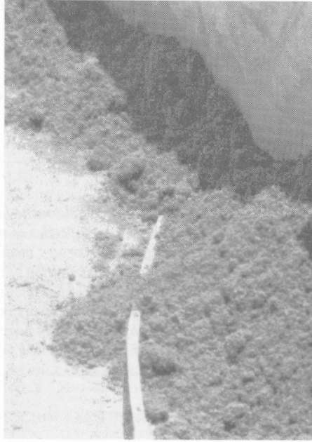
Fig 4 Wet sand is used to seal off the plastic sheeting on the concrete floor. In the foreground is the nylon tubing that is used to apply the methyl bromide in the evaporation pan.
