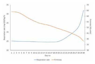
**Figure 11.** Example of the relationship between the respiration rate and firmness reduction rates of avocado fruit over a one month storage period.
