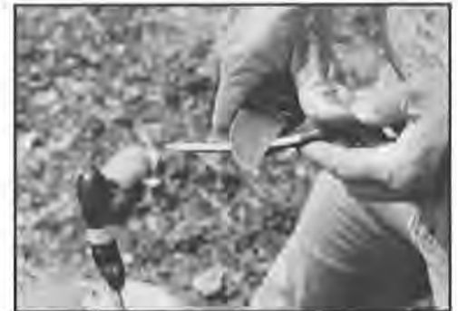
Fig. 24. Cutting the flat wood-side taper (notch at upper end is optional).
