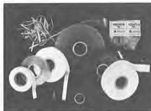
Fig. 5. Various polyvinyl plastic tapes, as well as wrapping rubbers (upper left) and wrapping film (upper right).
